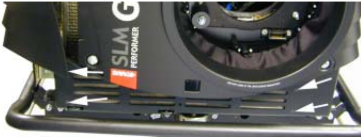
Image B-4 Dust filter removal
